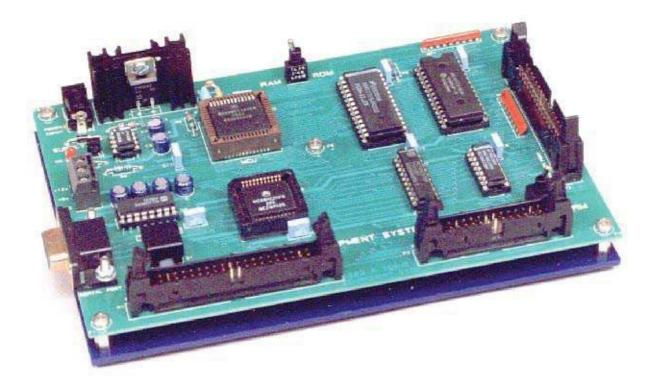
The 24-102 68HC11 DATS is a single board computer based on the powerful and popular Motorola MC68HC11 micro-controller unit. This highly flexible product is designed to be used as a development system and training aid or as a stand-alone controller or computer.
