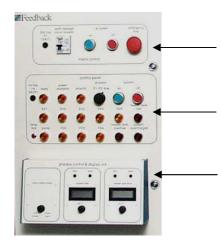
Area one houses the main ac power control that includes separate power on and off push-buttons, emergency power off button and supply earth leakage breaker.
