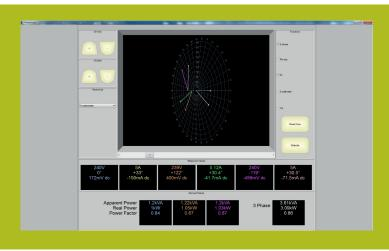
When operated in conjunction with the new 67-505 Swinging Field Dynamometer and the new 68-445 Machine Testing System, data can be taken from both systems simultaneously so plots such as torque against power factor may be created.
