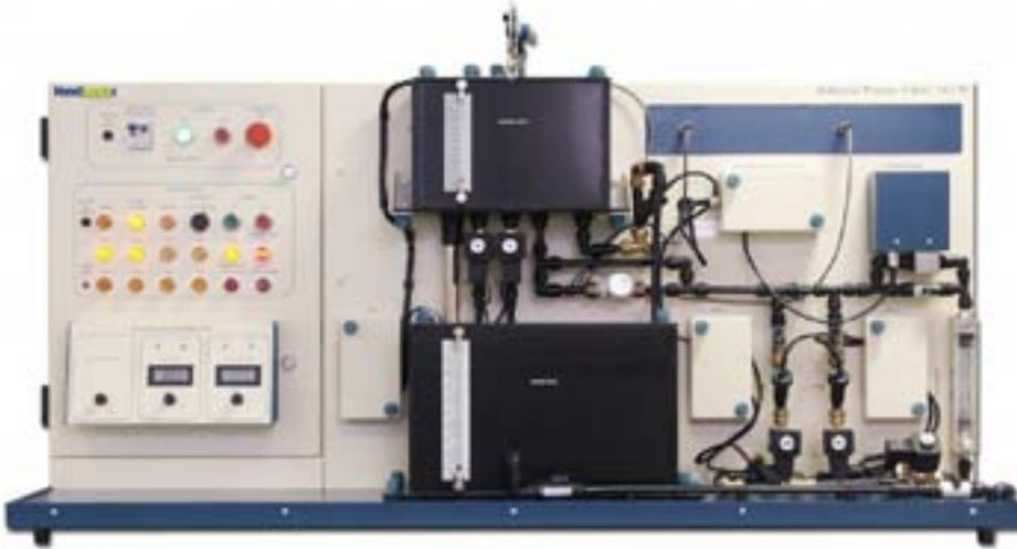
The Industrial Process Trainer has been designed to teach a methodical approach to fault diagnosis in industrial processes. The methodologies taught within the system are equally relevant to any student or trainee studying fault diagnosis. Faults can be introduced by the instructor via switches concealed behind a locked compartment, to which the student does not have access.
