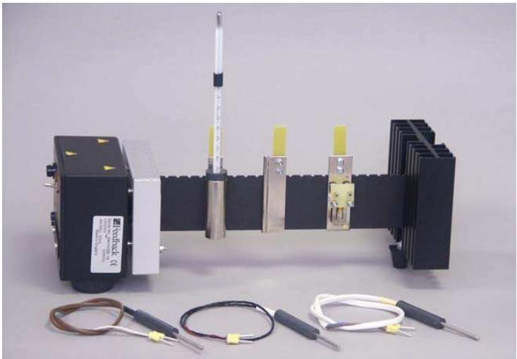
The test mount for the temperature transducers consists of a heat bar. This is equipped with a heater at one end and a multi-finned heat sink at the other. The temperature gradient produced along the bar is utilised to explore the characteristics of a number of transducers. These are attached to the bar in the desired position by a clip. Calibration is achieved by means of mercury in glass thermometer dipped into a water tank which may also be clipped to the bar.
